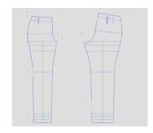
Drawing - 1. Drawing of a basis of a design of trousers (170 - 48 - 39,5)
